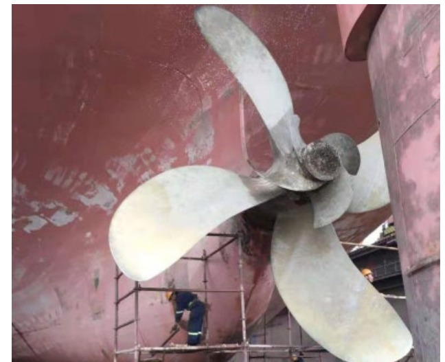
Propeller boss cap fin on M/V PEDHOULAS ROSE
