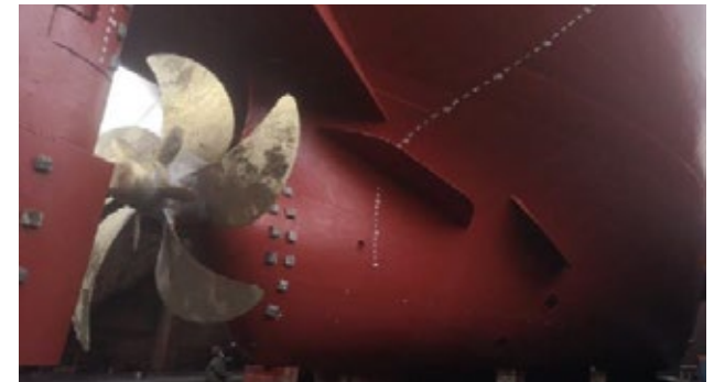
Duct and propeller boss cap fin on our newly acquired vessel M/VKOULITSA 2
