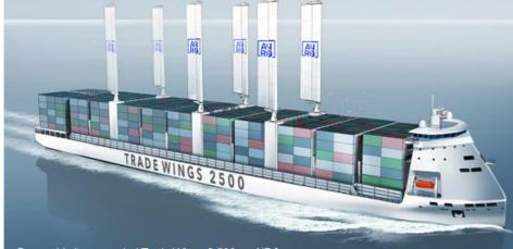
Bureau Veritas awarded Trade Wings 2,500 an AiP for its combination of Oceanwings® wind-assisted propulsion technology with LNG-electric propulsion. © Copyright SDARI, AYRO, VPLP Design, Alwena Shipping
