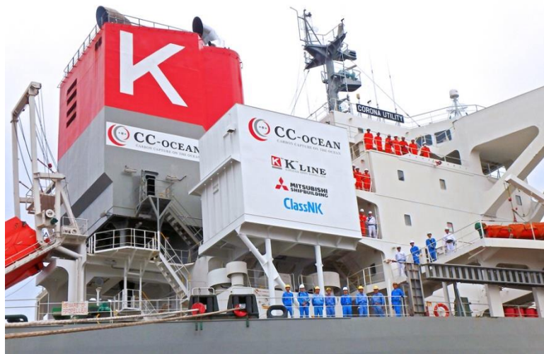
Marine-based CO 2 Capture System installed on board the CORONA UTILITY
