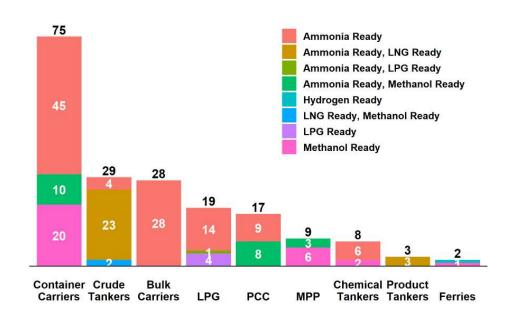
Alternative Fuel Ready of choice is LNG... with emerging alternative fuels... Ammonia and Methanol (container carriers)
