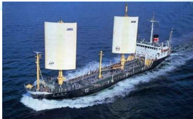
Sail-assisted tanker “SHIN AITOKU MARU”(1980)
